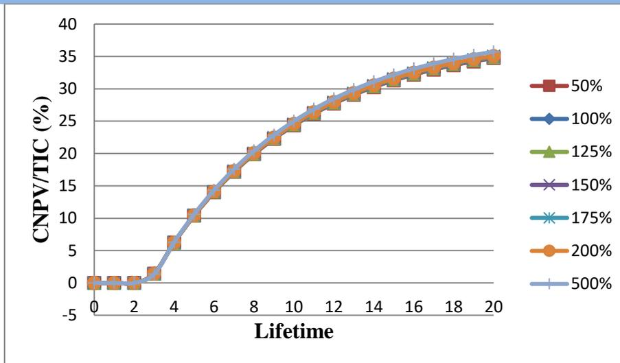
Figure 8. The effect of the number of workers on CNPV/TIC for 20 years.
