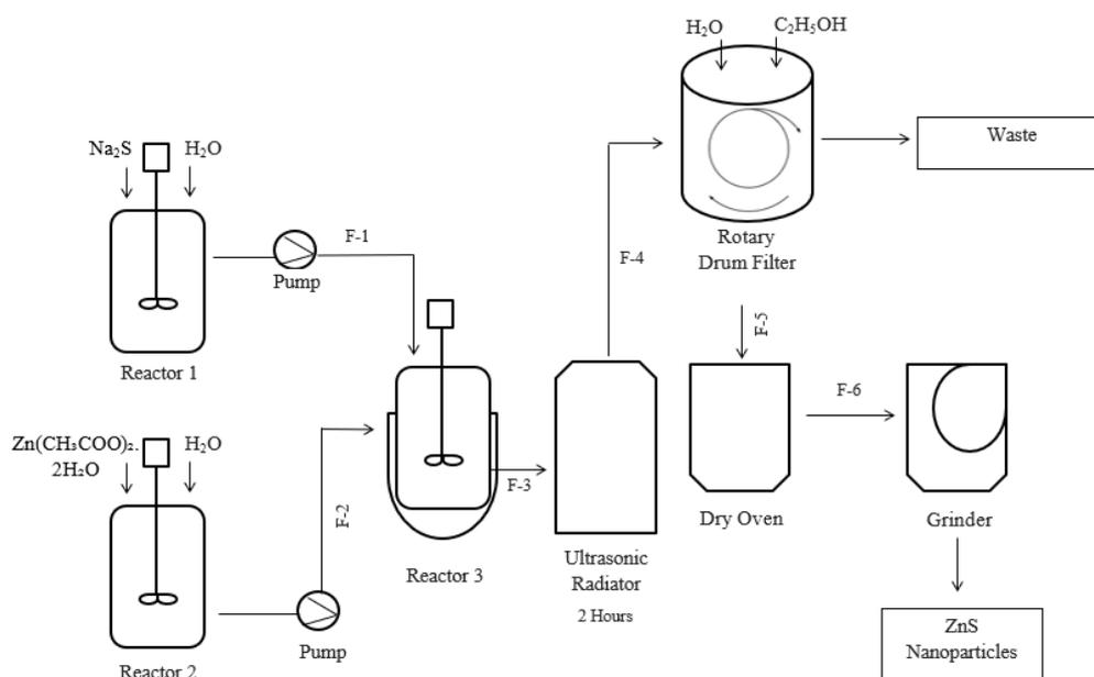
**Figure 2.** Process flow diagram on the production of zinc sulfide nanoparticles.
